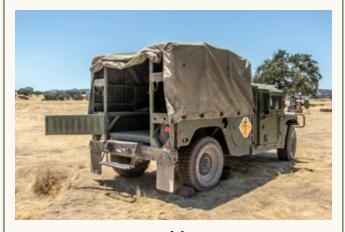
The HUMVEE **Ammunition Support** vehicle provides enhanced safety capability and functionality to soldiers supporting artillery units. It provides artillery crews improved seating and seat restraints, crush protection of 10,000 lbs., a flexible payload configuration, and its design simplicity allows for a small logistic footprint.
