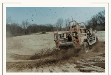
The **Troop Transport (9)**, installed on the HUMVEE 2-CT<sup>™</sup> platform, is a 9-soldier conversion kit with crush protection of 10,000 lbs., improved seating and integrated restraints, a 360° weapons ring, and available mountings for squad weapons.
