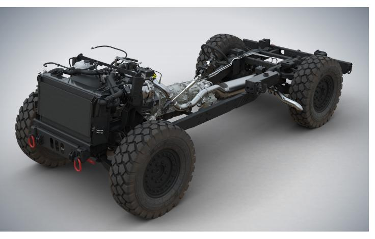
The Multi-Purpose Truck (MPT) Powered Chassis is a commercial base, 4x4 platform truck chassis engineered to serve the extreme environment needs of energy, mining, industrial and government customers around the world. The MPT chassis is available as a fully assembled rolling chassis (complete frame, powertrain and driveline) ready for adaptation to a variety of cab and body configurations or as a knockdown set of components which can be customer assembled.
