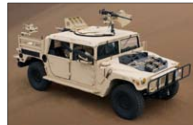
M1165 HMMWV with B-kit removed, reconfigured as Special Operations HMMWV.
