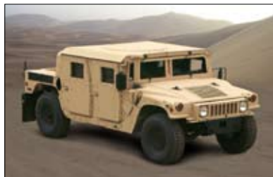
M1165 HMMWV with A and B field installable/removable armor kits.
